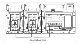
Each EXP40 expansion module provides you with 20 EXP keys and 2 display pages, supporting a total of 40 EXP keys that you can set up as contacts. You can connect up to 6 EXP40 expansion modules to your phone to support a maximum of 240 EXP keys per phone.
