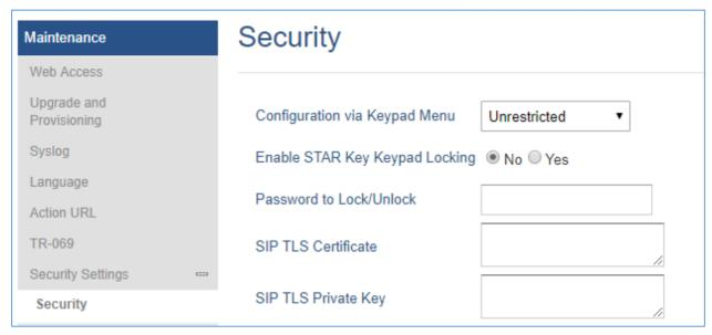
Figure 3: Lock/Unlock Configuration via Keypad Menu
