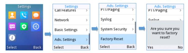
Figure 14: WP810 LCD - Confirm Factory Reset
