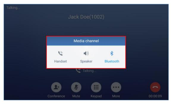
Figure 53: Switch Audio Channel during Call
