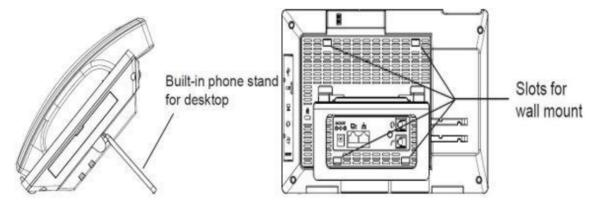
Figure 5: Built in Stand and Mounting Slots on GXV3380
