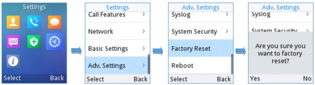
Figure 57: WP810 LCD - Confirm Factory Reset
