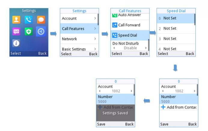
Figure 34: Speed Dial Configuration
